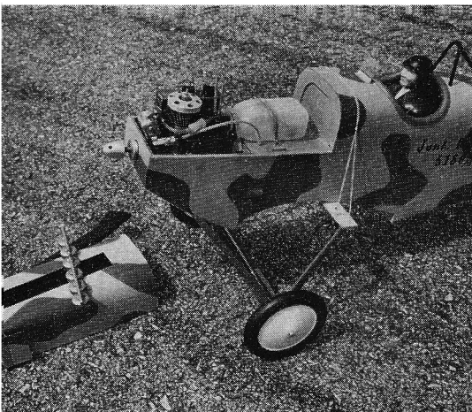
With the top hatch removed, a neat arrangement of engine, tank, etc. becomes evident.
