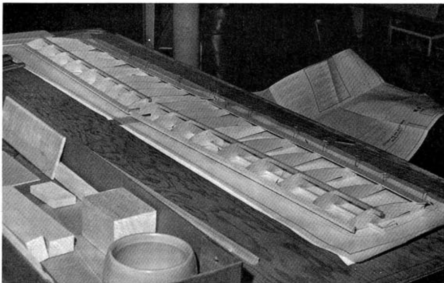
The bottom wing spar and ribs are pinned to the building board through the plan, then the leading and trailing edge parts are added.
