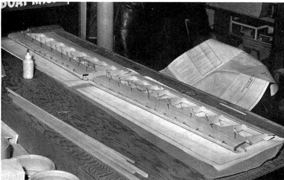
Most planking has been glued to the wing. Next, the wing halves will be trimmed, sanded, and joined together.
