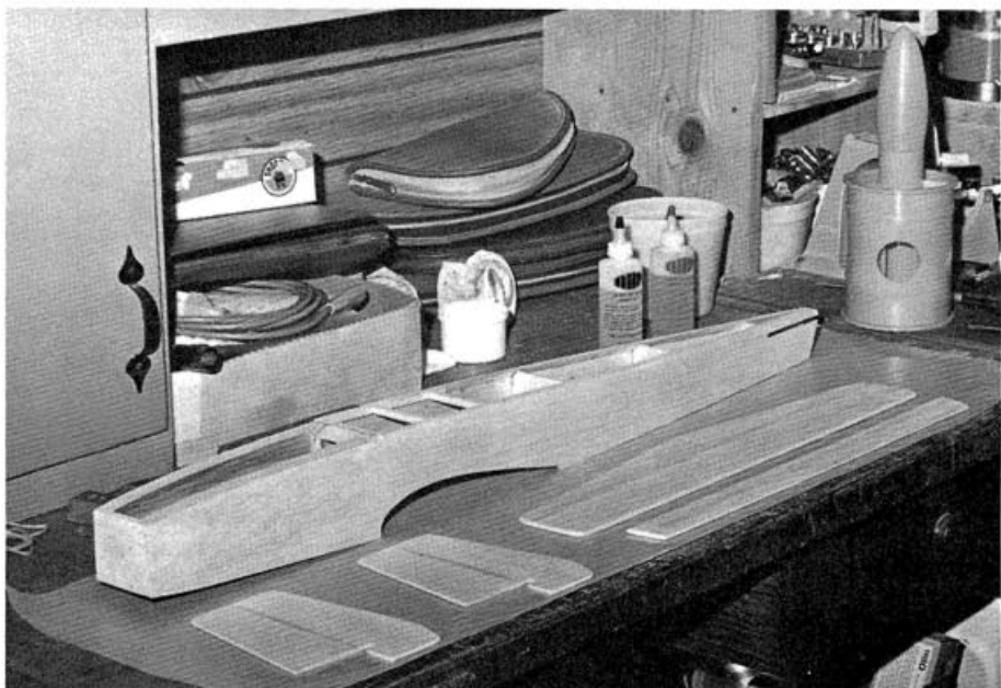
All bulkheads have been installed in the fuselage and the sheet balsa tail surfaces have been assembled and sanded.
