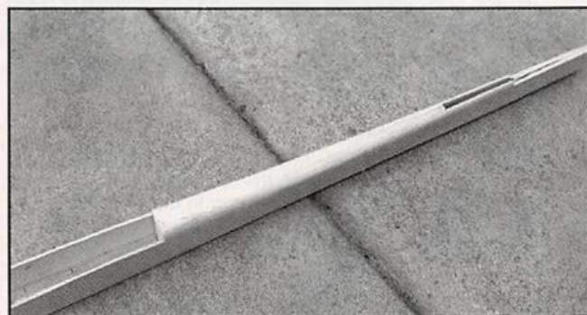
Rear of fuselage shaped and sanded, then slotted for the vertical fin and stabilizer.
