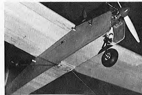
Above: Tail assembly before covering with Silkspan. Surfaces are squared off to reduce tedious details. Fin is permanently attached, stabilizer is held on with rubber bands to minimize damage. Top, right: Installation showing Enya 09, Sullivan SS-3 tank, battery and radio compartments. Clyde the pilot is ready to go aboard. Right: Portrait of the classic tricycle gear which insures straight tracking and easier piloting technique on both takeoffs and landings.
