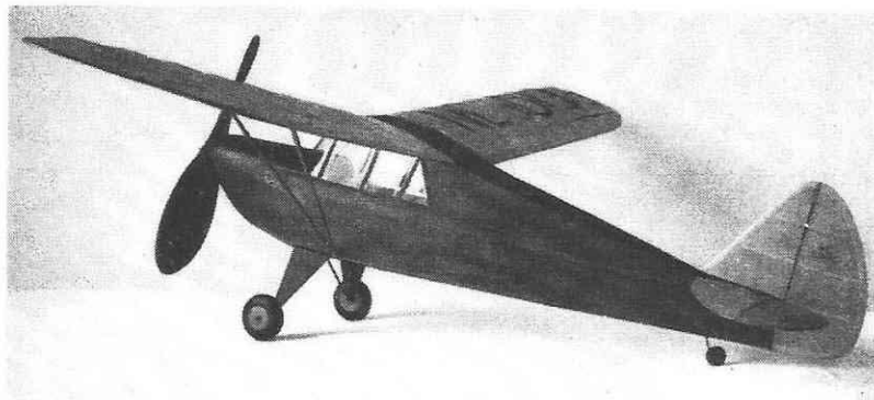
Stability from high wing; efficiency from large prop
