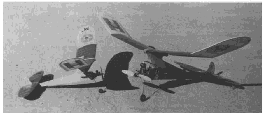
Jerry Murphy enjoyed the .020 Replica version so much, that he built a full-size model of the Class B ship and installed his old K&B ignition .29.
