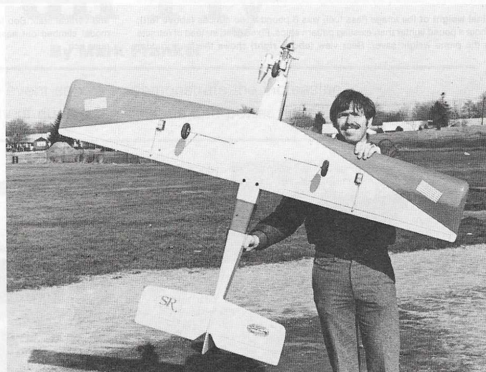
Grumman Aero Test engineer, Tom Hunt, holds the Image up to give you a view of the underside. Note the position of the aileron servos. This method allows such easy access and adjustments. Becoming quite common.
