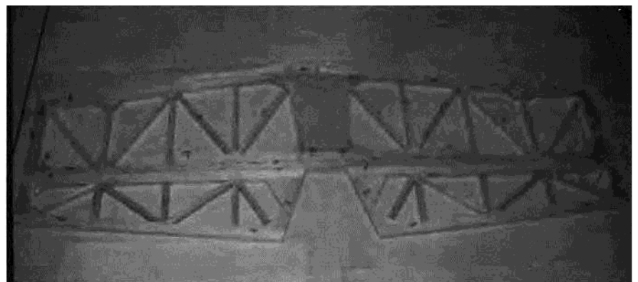
Horizontal stabilizer and elevators also use stick construction.
