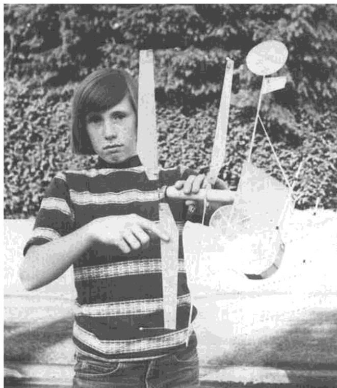
Roy's son Bob shows how to hold the 'copter for hand winding. It can also be winder wound from top end. Plug removable.
