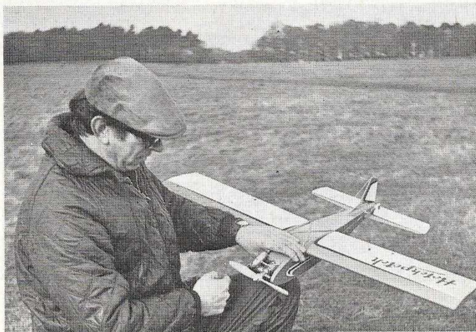
Original Hotchpotch had a diesel installed—easily started on the knee, as demonstrated by designer Ken Murgatroyd. Below: now has glow engine.
