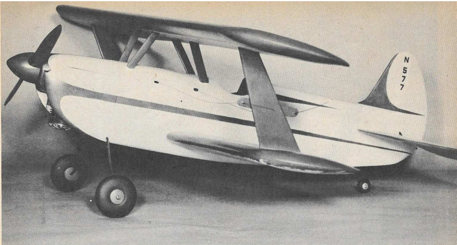
Big advantage of the biplane is small overall length necessary to get the tail where it belongs in relation to the wing, a fact which explains the
