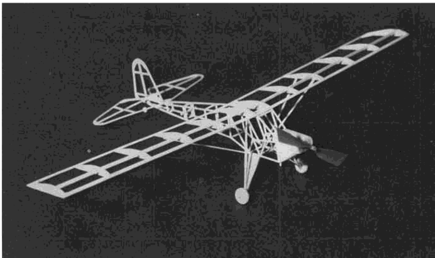
By using 1/20- instead of 1/6-square sticks, the weight was kept to a minimum for indoor flight. Covering was pre-shrunk and decorated condenser paper.
