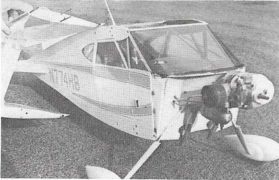
One of the things that causes the most head-scratching by builders from plans is the engine installation, as very few designers seem to provide photographs of their models without the cowl! The three views here, then, should make the arrangements pretty explicit. The top one, plus that at right, also shows wing fixings.
