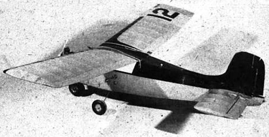
Rear quarter view clearly shows elevator and rudder areas and the arrangement of the control rods. Pins on both surfaces may be moved to alter movement. Wheels are barely behind CG position.
