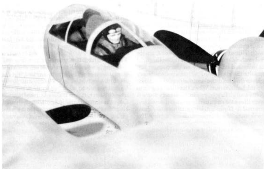
The acetate canopy for the cockpit was formed in two sections (above). It was first heated, then stretched over the canopy plugs. You won't need much more than the tools shown (below) to build the Uhu .
