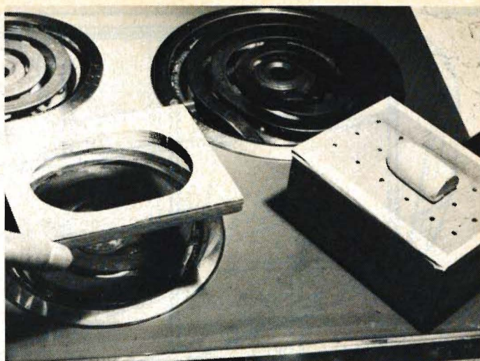
The plastic film is warmed until it is sagging, then positioned over the canopy, in contact with the lower box. It solves many a modeling problem.
