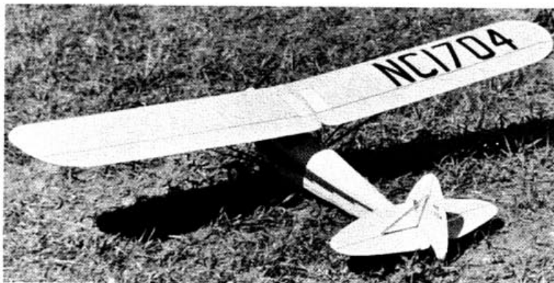
Sometimes scale has its advantages; here, the long wing of the Heath produces smooth turns and nice recoveries. The weight including the .099 engine is just 40 oz., ideal for RC original design.
