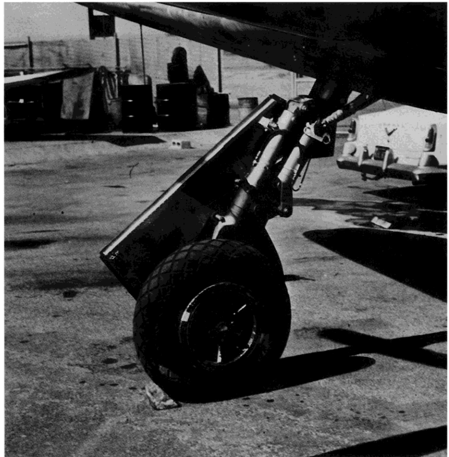
A detail view of the right main landing gear on a Sea Fury. Gear had to be beefy to handle such a heavy airplane during carrier operations.
