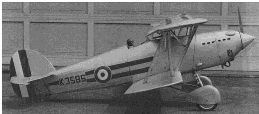
Profile view of the Hawker Fury reveals streamlined fuselage shape, wheel pants (which were not found on the Mark I version), and lightweight tail structure. Quadra powered.
