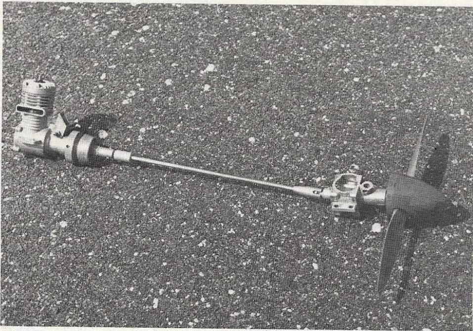
General hardware components. Fox .35 powerplant, Octura boat hardware and an old engine crankcase. Beneath: All connected up. Engine electric starts with a v-belt. Bearing needs some lubrication.
