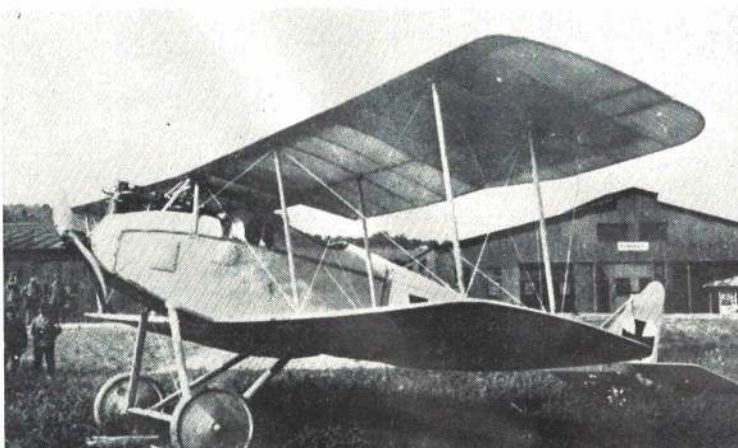
Of interest here are the rigging wires, fuselage inspection panels, and cabane struts. Right: Camouflage typical only on the Baron's plane.
