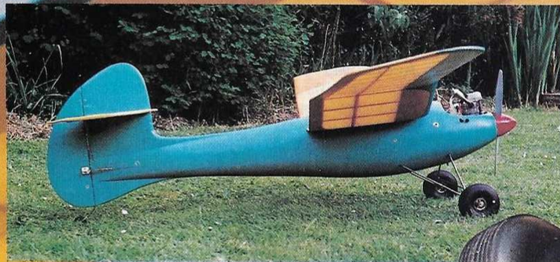
Classic fuselage lines achieved with simple balsa planking.
