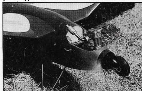
Gullable takes any .20 to .25 motor; prototype flies well on a .20 four-stroke.
