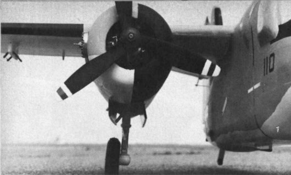
Build two nacelles, that's enough. Lengthy hardwood engine mounts form basis, formers, planking. Six J-boits secure each landing gear. Three-bladed props add realism, as does the gear detailing.
