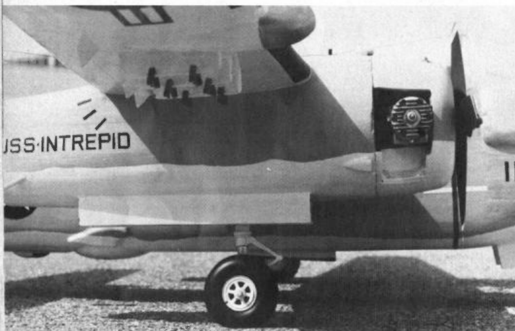
The bomb racks are visible here on the underside of the wing. Gear doors are of 1/8" sheet. Keep weight within reason, balance on the C.G. Aircraft flies well, but wait for a reasonable day. Below: Tail surfaces. Dual elevator pushrods are required due to the dihedral of the stabilizer.
