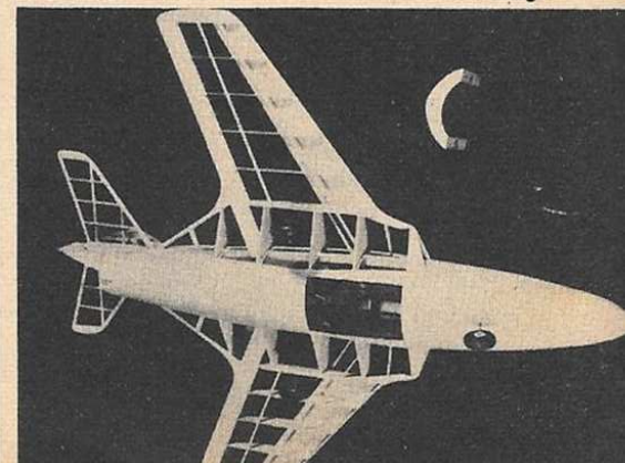
Bottom view shows air recess opening in belly. Opening is covered with an aluminum screening.
