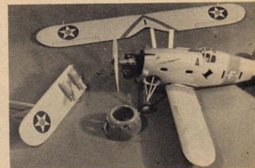
Big feature of design is complete break-away of major components, minimizes the splinters.
