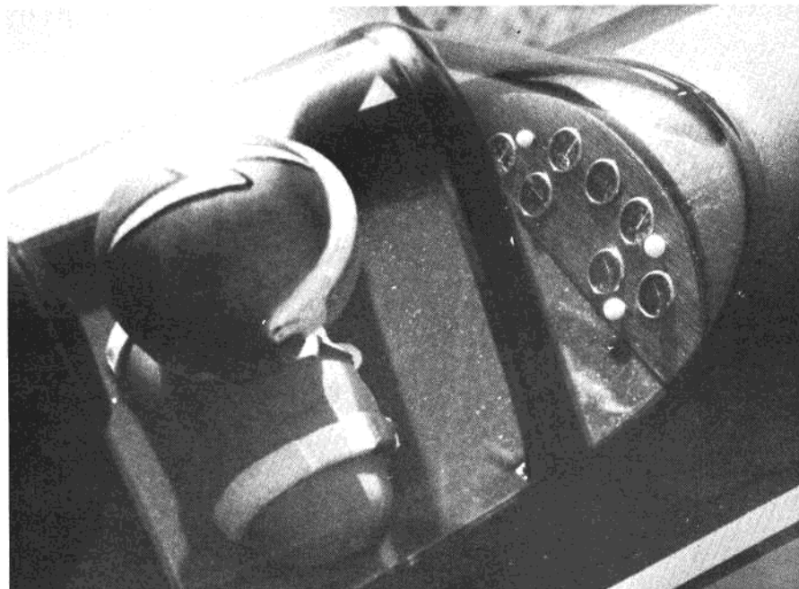
Cockpit details always attract attention and make a non-scale model look real. Interesting here is the use of a plywood canopy for handling strength.
