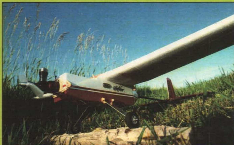
This ground-level close-up clearly shows the Grasshopper's rubber-band-together assembly. Dave used MonoKote on the fuselage pod and tail surfaces. Pod could also be painted with K&B Super Pox for a durable, totally fuelproof finish.
