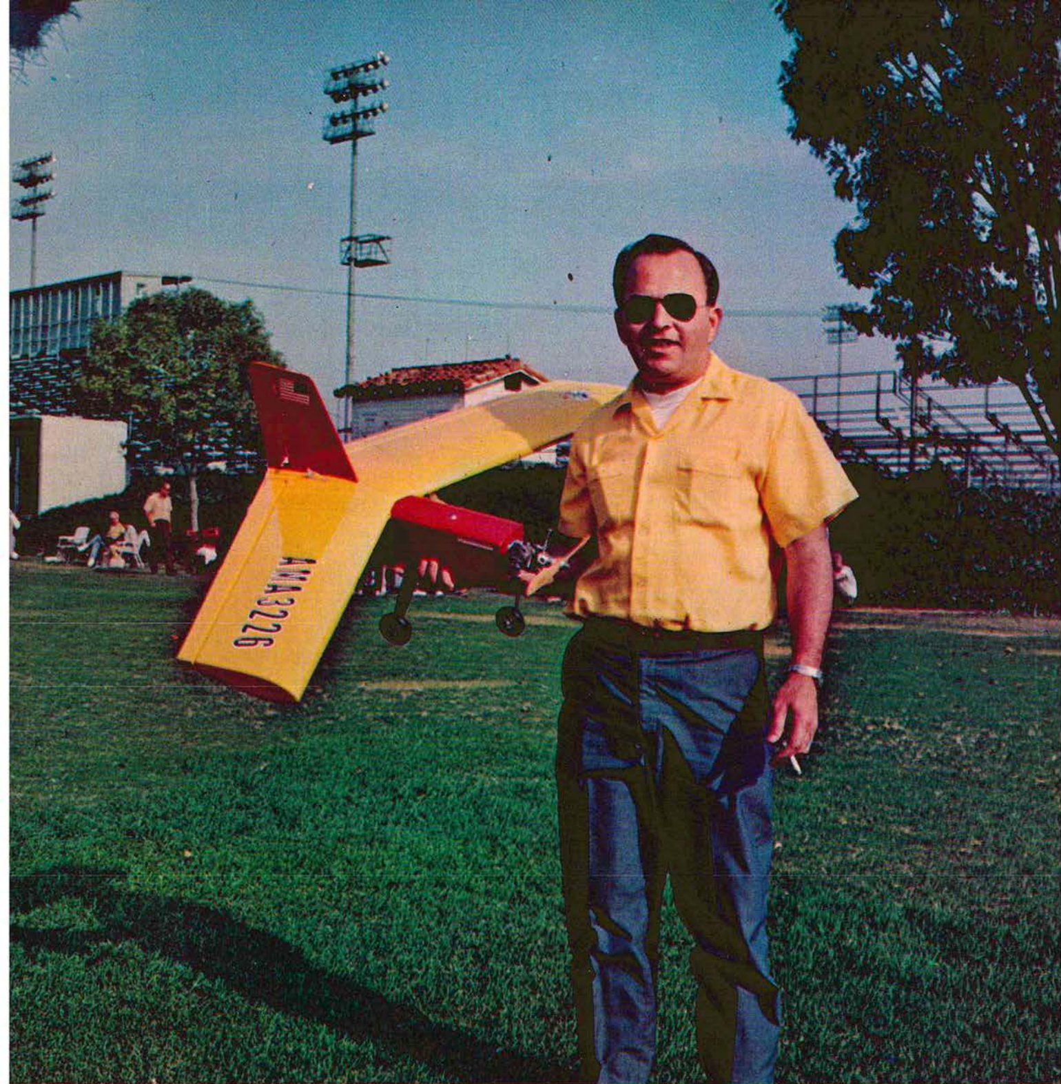
RCM's Technical Art Editor, Dick Kidd, displays unusual appearance of the Goose. MonoKote covered, Enya .29, Micro Avionics proportional system. Ektachrome by Don Dewey.
