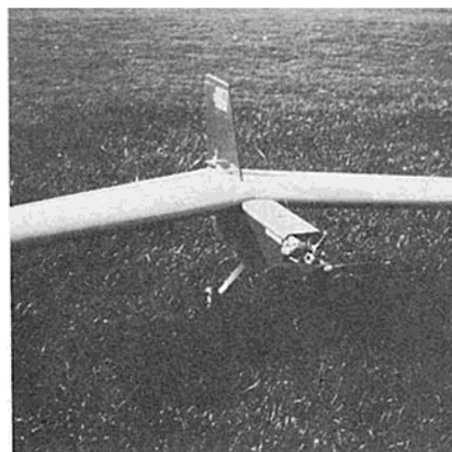
The Goose at rest. First flight on RCM prototype near-disastrous due to improper incidence, requiring excessive up-elevon trim.
