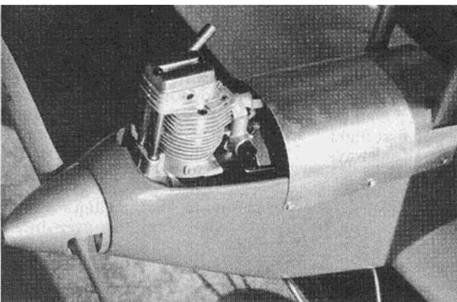
Removable aluminum tank cover made from aluminum roof flashing from building supply. Engine is O.S. FS-40 four cycle.
