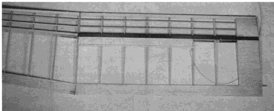
Wing structure follows standard practice; only unusual feature is that bottom of l.e. is sheeted, top is not. This particular wing uses experimental carbon spars, recommended for FAI.
