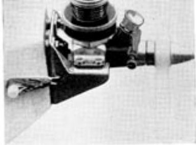
Above: close-up of Cox TD049 power plant on knock-off dural mount. Correct thrust line obtained by packing out with washers. Right: Go-jet from the rear. Fast model requires quick reactions.
