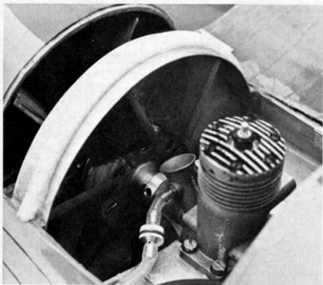
ABOVE: The heart of the matter is the fan system. The author has been working with DFs for a long time to learn how big, how many fans, what airfoils, etc. The installation is like a pusher's. LEFT: Your happy author holding his plane illustrates that this is a big model. By the way, the real plane also has a smooth skin since most of it was plywood-covered.
