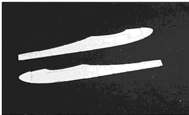
The completed fuselage sides.
