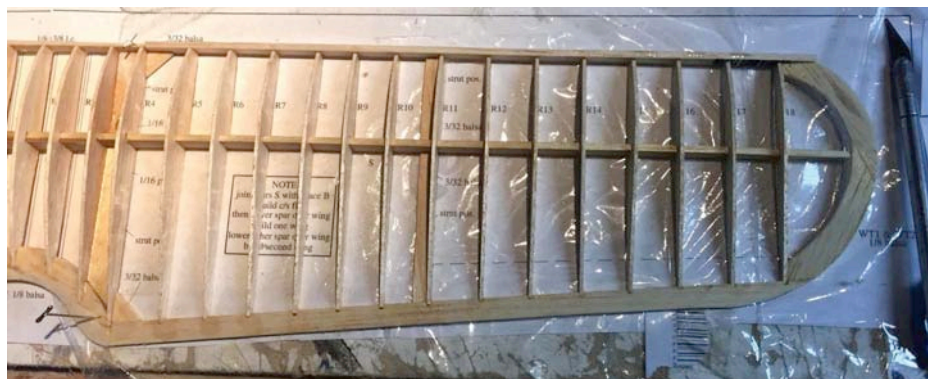
The spar is lowered over one wing panel and the panel assembled around it.
