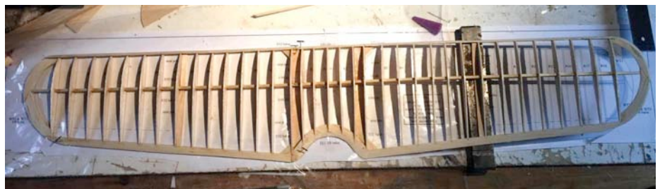
Finally the built side is packed up while the second wing panel is built.
