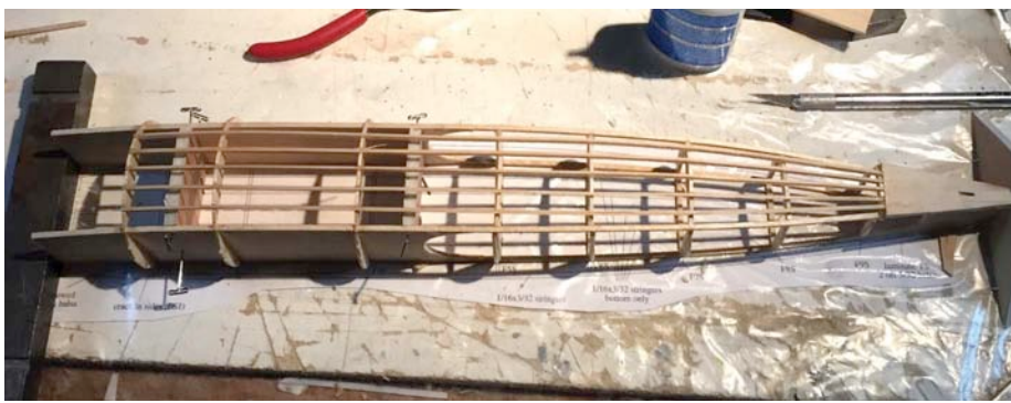
Although not quite the order in which I described, this shot demonstrated how the entire fuselage can be braced (pinned down) while formers and stringers are added.
