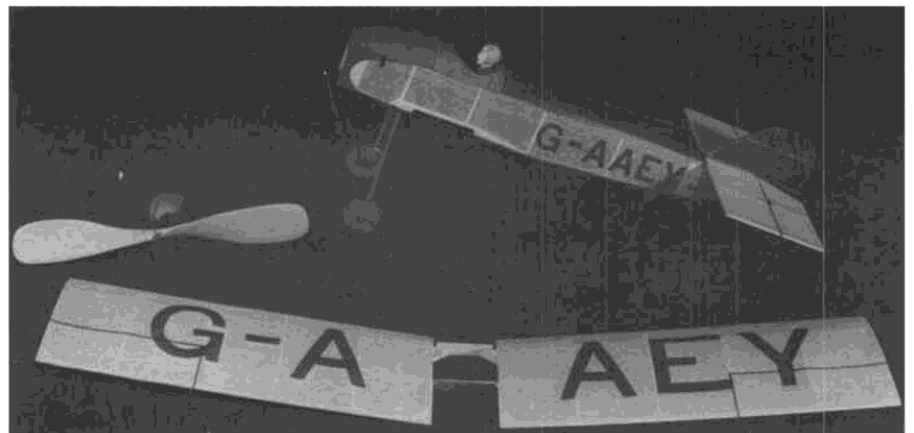
The Gadfly disassembles for shoe-box transportation. Wing is friction fit into fuselage.
