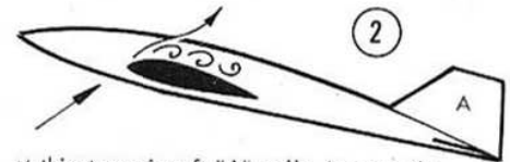
at this stage aircraft "A" stalls, because the airflow no longer flows across the top of the wing
