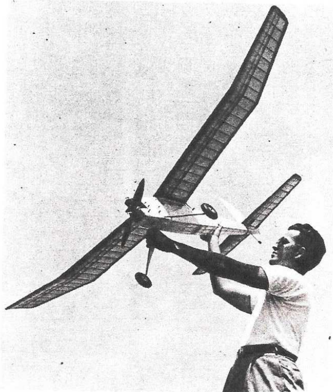
The wingspan is eighty-four inches, giving a smooth, flat, consistently good glide. Although the author used an ignition engine in the original, any glow-plug engine, from .29 on up to .61, can be used in the ship.
