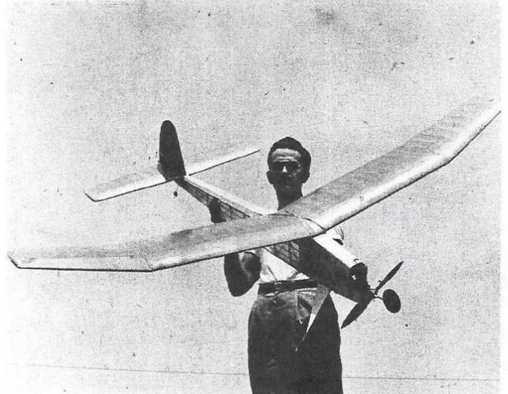
The finished product gives realistic performance as well as beauty. The details for the dethermalizer are described on the plans. Although the original was powered with a Super Cyclone, smaller engines can be used.
