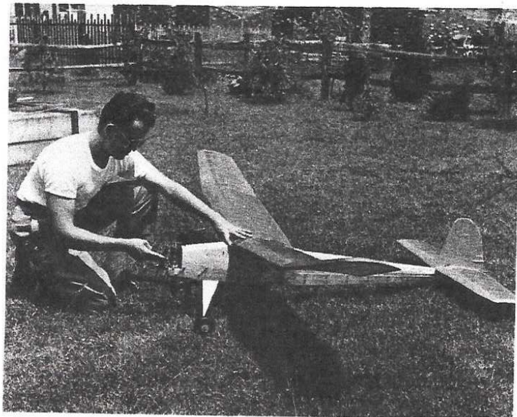
Airfoil is the N.A.C.A. 6409. The sheet planked leading edge assures retention of the proper airfoil shape. Note the long tail moment arm, polydihedral wings, and the wide, well-forward landing gear for good takeoffs.
