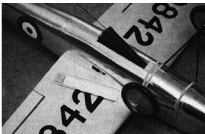
Inserting the drive battery. Note bands for landing gear.
