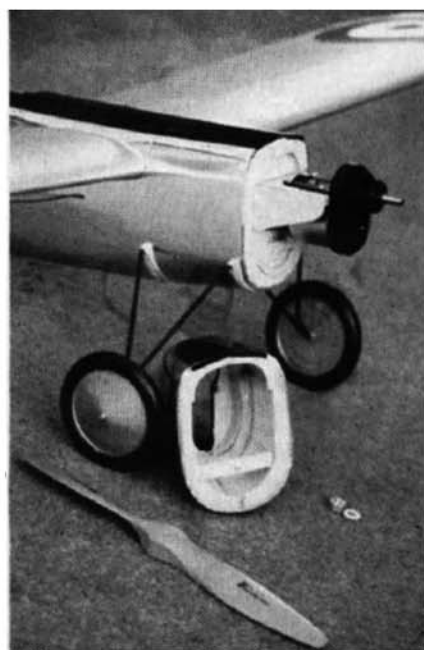
Power house. MFA RX 15 and Olympus belt reducer.
