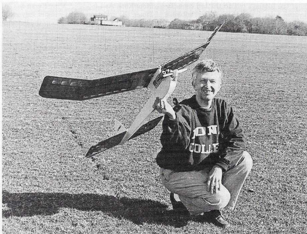
Bob poses with his modern Frisco Kid which nearly duplicates the same scheme as John Tatone's original. Final weight of Bob's Kid came to 32 ounces for a very light 10 ounce/square foot wing loading.
