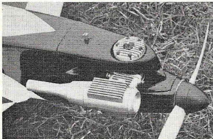
Close-ups show the speed-type cowling and the upright installation of the rear-induction K & B.
