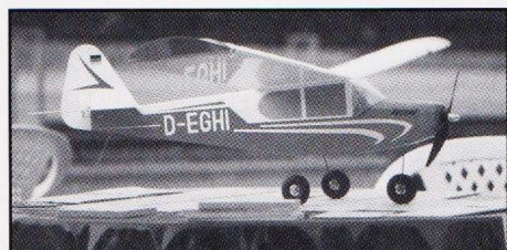
This view from the right side shows off the dihedral angle of the wing, which gives the model much of its stability, making it a good trainer. Because of its clean lines and finish the Frechdax looks very much like a sport aircraft.
