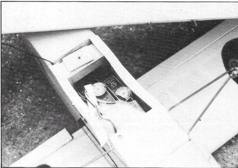
Above, access to the servos is via the lower wing opening, while the receiver can be reached through the upper wing housing.
