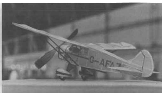
Ship has nice proportions for stable flight, and the long scale landing gear and high thrust line allow a generous size propeller.
