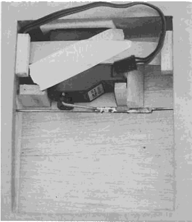
Aileron servo sits on foam pad and is restrained by scrap balsa box — works!
