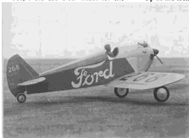
Not an easily mistaken shape! Generous wing and tail areas plus long moment arm gives good flying manners, too.
