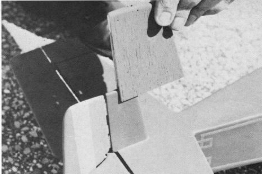
A good idea for a lot of test flights, as the scale rudder fin is very tiny to say the least, an enlarged fin was built with a slot within. It just slips over the scale fin for test purposes. One pin retains it. No stability troubles were encountered, but be wary in slow-flight range to be sure.
