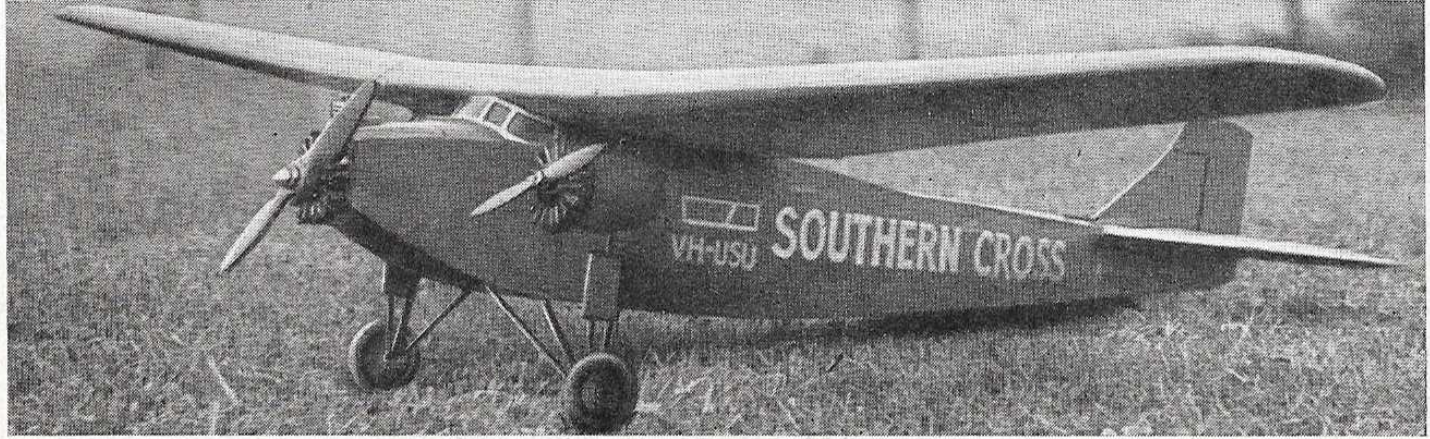
The unusual thick wing of the real F.V11b is a great help for scale free-flight, providing a realistic flying speed with the Kalper power.
