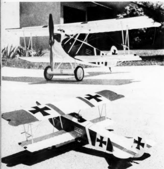
Both D-7's are precise scale, including the paint schemes. Machine guns, visible in rear view, are built up of sheet brass and wood; are removable.
