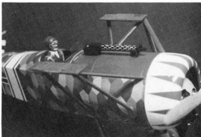
LEFT: Forward hatch removed. Hold-down is by long bolt through dummy machine gun mount which screws into blind nut in cross member above fuel tank. RIGHT: Both hatches in place. Note dummy machine gun as on Sweringen's replica. Twin Spandau guns were used on standard D-VIII's, and are available from William Bros.
