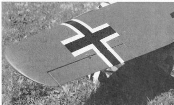
LEFT: Close-up of wing top detail. Note reinforcing tape and dummy aileron horn and rods. RIGHT: Close-up of tail surfaces, showing dummy horns and cables.
