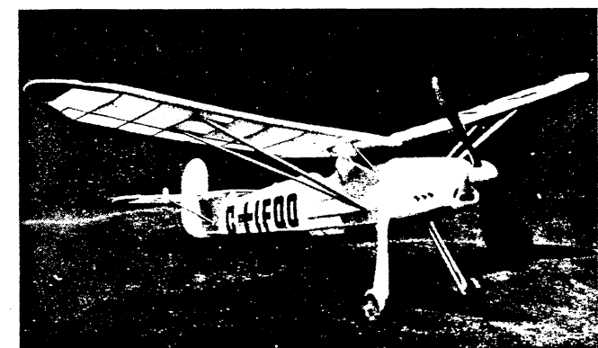
The parasol wing and forward-mounted stabilizer, that are peculiar to this ship, can be seen here. The design is well suited for model work.
