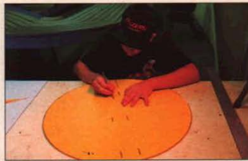
Cutting out the slots for the fuselage tabs and rudder tabs.
