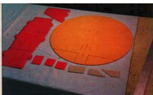
Floppy Disc parts layout. The only wood parts are the plywood firewall, side doublers and front bottom doubler.
