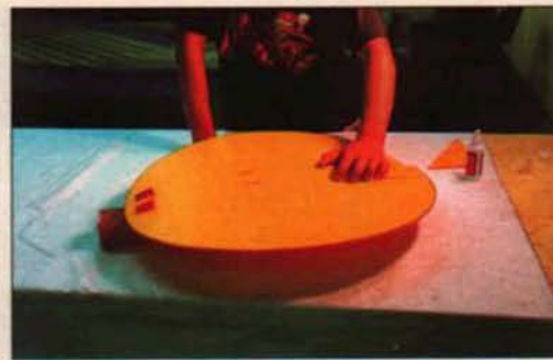
The wing is inserted over the fuselage tabs and glued with CA (author finds that Polyzap gives the best results).
